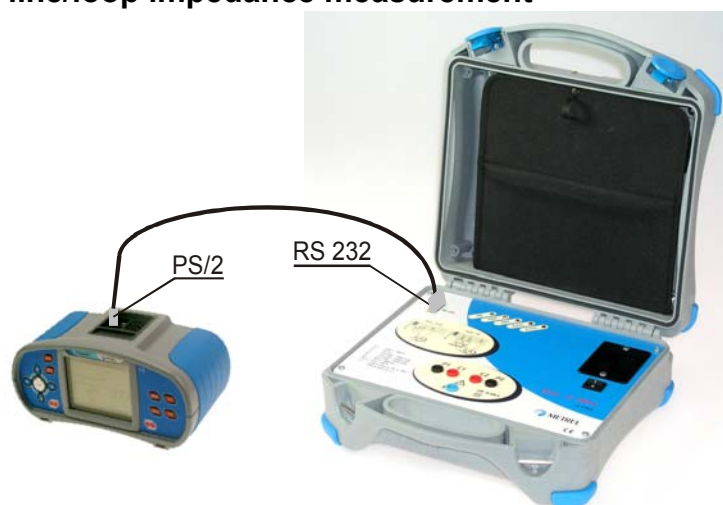
Figure 5.55: Connection of impedance adapter to the instrument
